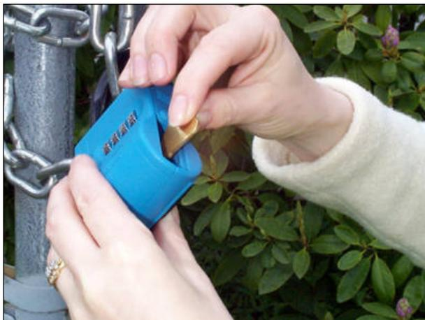
After sliding the door up to the key compartment they then retrieve the key.
